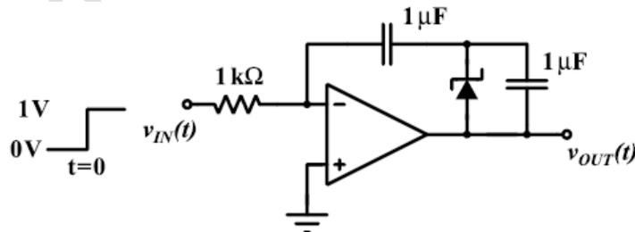
The time  $t$ , in milliseconds, at which the output voltage  $v_{OUT}$  crosses  $-10$  V is
