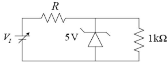
The value of  $R$  and the minimum required power dissipation rating of the diode, respectively, are
