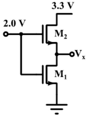
The voltage (in volts, accurate to two decimal places) at  $V_x$  is \_\_\_\_\_.
