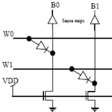
During the read operation, the selected word line goes high and the other word line is in a high impedance state. As per the implementation shown in the circuit diagram above, what are the bits corresponding to  $D_{ij}$  (where  $i = 0$  or  $1$  and  $j = 0$  or  $1$ ) stored in the ROM ?
