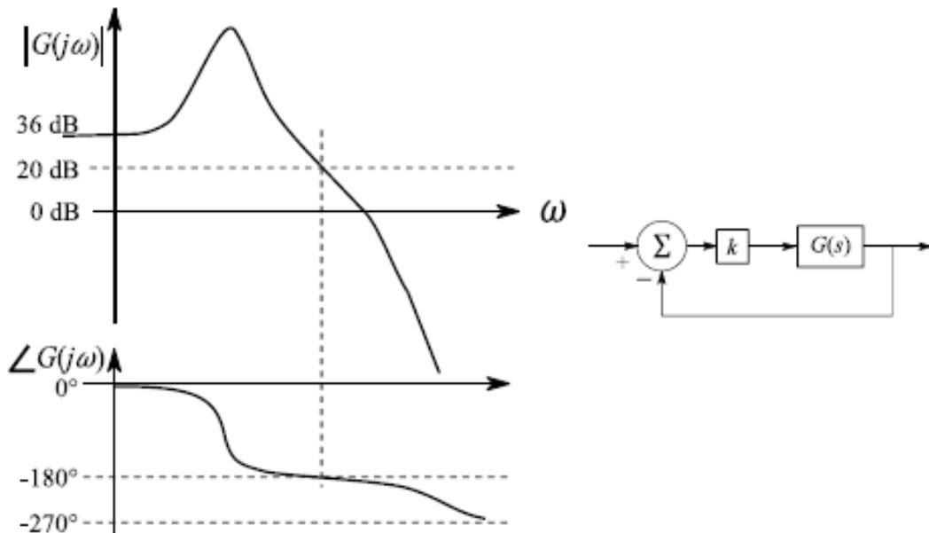
Consider the negative unity feedback configuration with gain  $k$  in the feed forward path. The closed loop is stable for  $k < k_0$ . The maximum value of  $k_0$  is \_\_\_\_\_ .
