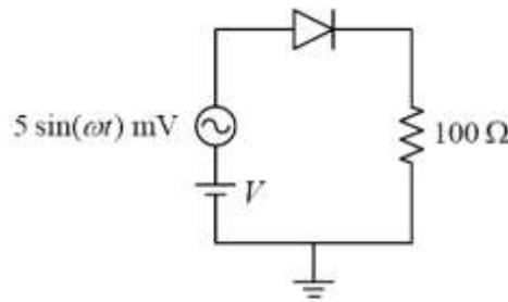
For  $\omega = 2 \times 10^6$  rad/s, the amplitude of the small-signal component of diode current (in  $\mu\text{A}$ , correct to one decimal place) is \_\_\_\_\_.
